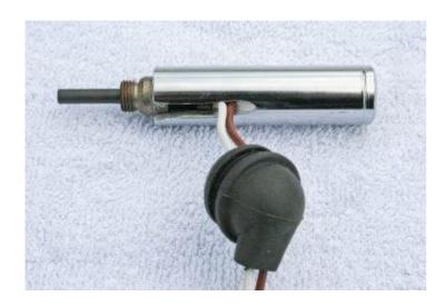
now reconnect your glow plug to the heater pcb (ensure it is clear of any obstruction as it will glow red hot if working ok) reconnect your supply to the heater and hit the start button
