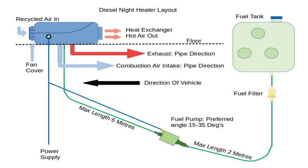
Fuel tank, pump, heater, fuel line lengths
